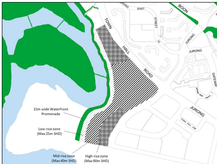
Fig 12 - Building Height Control Plan
